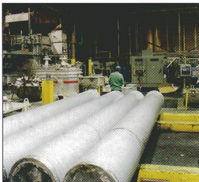
Figure 7. Larger diameter (675mm) alloy 7050 billets cast with LARS refining system. The SCADA control cabinet and HMI can be seen in the background.
