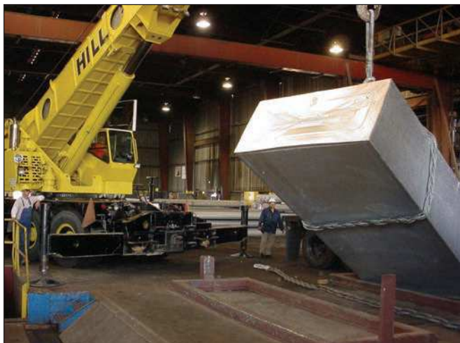
Figure 1. Vista Metals' 70,000 lb super slab being removed from casting pit.
